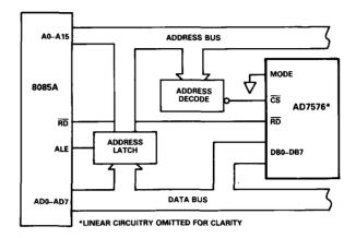
Figure 10. AD7576 to 8085A Asynchronous Conversion Mode Interface
