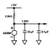
Figure 14. Reference Circuit
