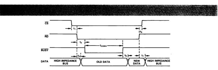
Figure 5. Slow Memory Interface Timing Diagram
