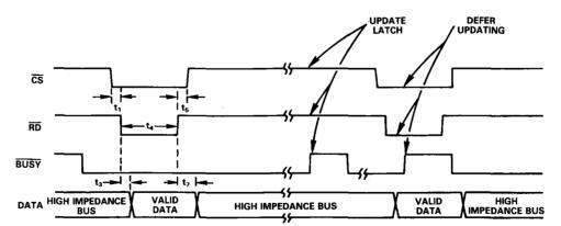
Figure 9. Asynchronous Conversion Mode Timing Diagram
