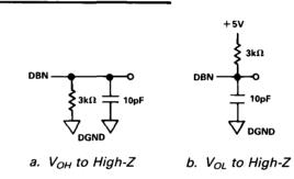
Figure 1. Load Circuits for Data Access Time Test
