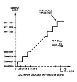
Figure 4. Nominal Transfer Characteristic for Unipolar Operation
