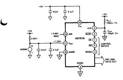
Figure 3. AD7576 Operational Diagram
