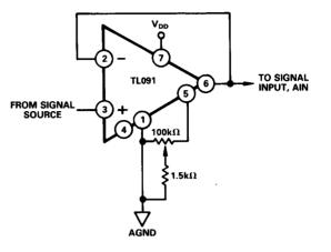
Figure 13. Offset Adjust Circuit
