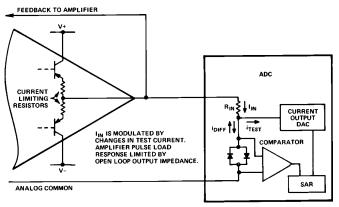
Figure 6. Op Amp—ADC Interface
