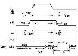
Figure 2. Read Cycle Timing
