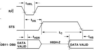
Figure 4a. Stand-Alone Mode Timing Low Pulse  $R/\overline{C}$
