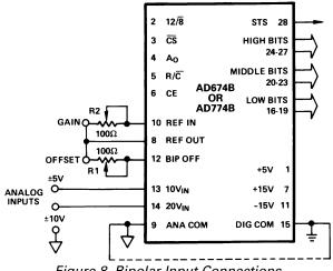
Figure 8. Bipolar Input Connections
