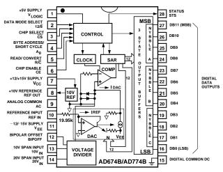
Figure 5. Block Diagram of AD674B and AD774B
