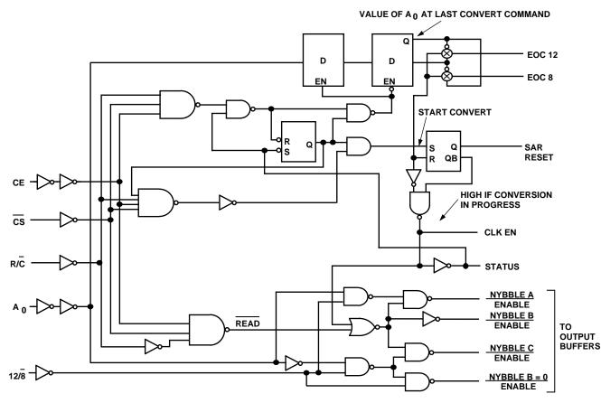
Figure 9. Equivalent Internal Logic Circuitry
