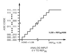
Figure 4. AD7992 Transfer Characteristic
