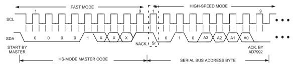
Figure 15. Placing the part into Hs-Mode
