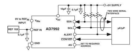
Figure 5 AD7992 Typical Connection Diagram
