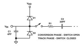
Figure 6. Equivalent Analog Input Circuit
