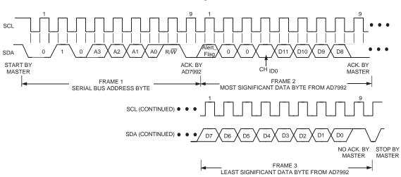
Figure 14. Reading two bytes of data from the Conversion Result Register
