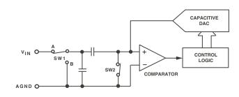
Figure 2. ADC Acquisition Phase
