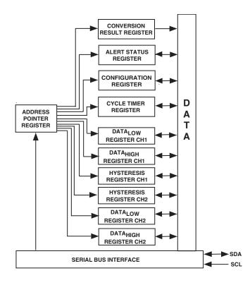
Figure 9. AD7992 Register Structure
