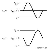
FIGURE 3. Expected Input Signal Range
