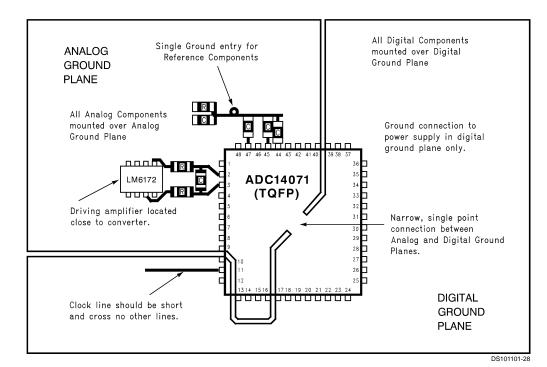
FIGURE 8. Example of A Suitable Layout
