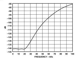
Figure 1. Noise Spectrum per 5 Hz (3.072 MHz Modulator Clock)
