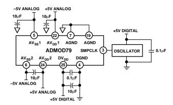
Figure 4. Recommended Bypassing and Oscillator Circuits
