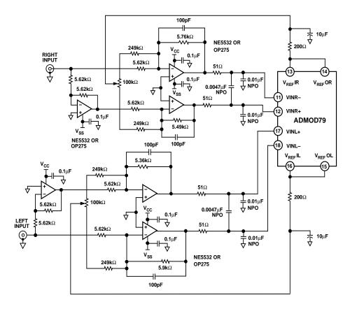
Figure 2. Recommended Input Structure
