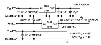
Figure 3. ADMOD79 Recommended Power Conditioning Circuit
