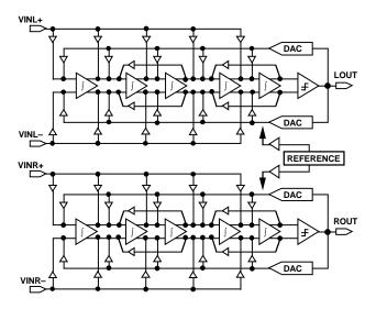
dynamic range and excellent common-mode rejection characteristics. Because its modulator is single-bit, the ADMOD79 is inherently monotonic and has no mechanism for producing differential linearity errors. Analog and digital supply connections are separated to isolate the analog circuitry from the digital supplies.
