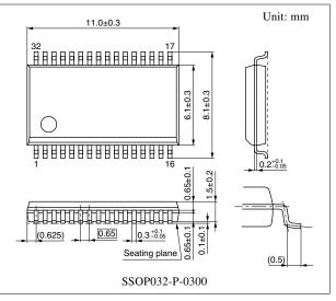
Note) The package of this product will be changed to lead-free type (SSOP032-P-0300B). See the new package dimensions section
