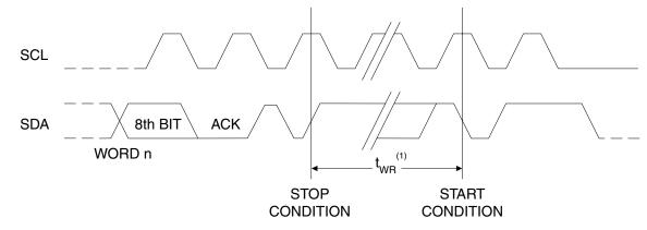
Note: The write cycle time  $t_{WR}$  is the time from a valid stop condition of a write sequence to the end of the internal clear/write cycle.
