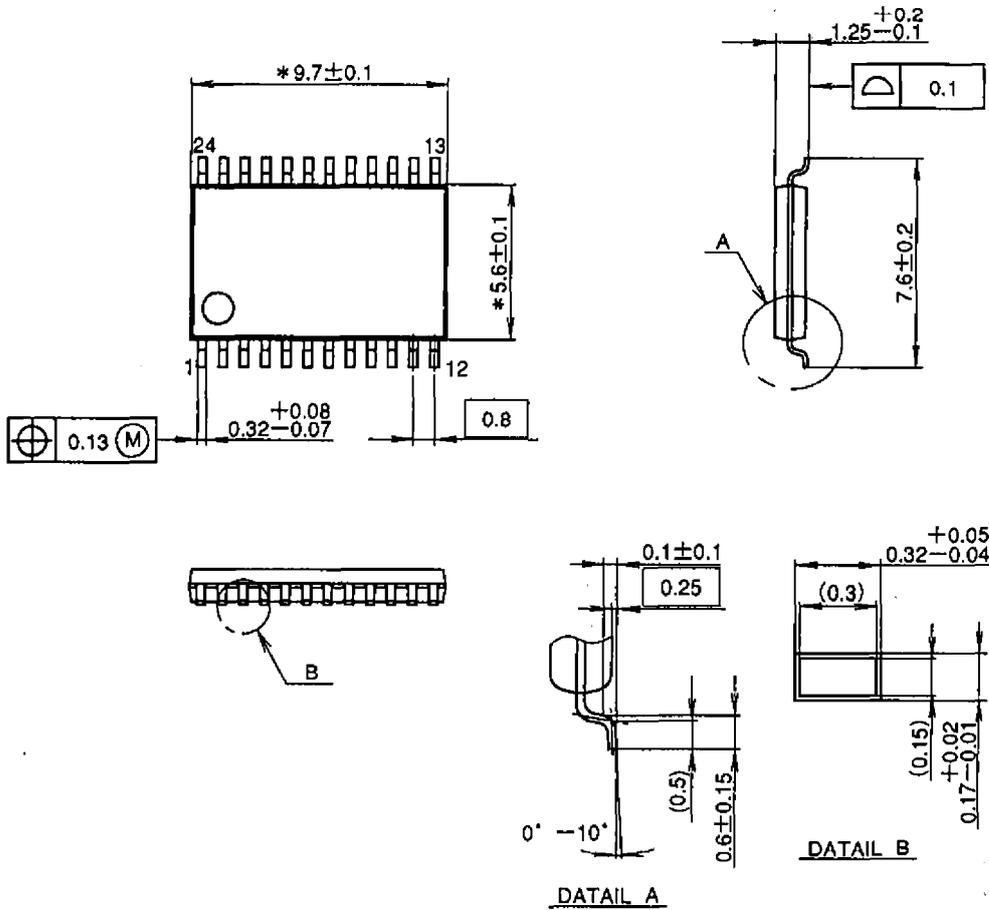
NOTE > "\*" Dimensions do not include mold protrusion.
