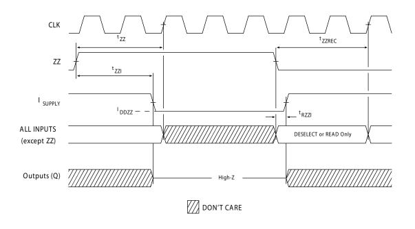
30. Device must be deselected when entering ZZ mode. See Truth Table on page 11 for all possible signal conditions to deselect the device. 31. DQs are in high Z when exiting ZZ sleep mode.
