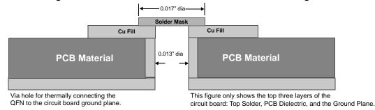
Figure 27. Plot of the Solder Mask (White Area)
