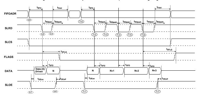
Figure 23. Slave FIFO Asynchronous Read Sequence and Timing Diagram
