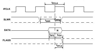
Table 28. Slave FIFO Synchronous Write Parameters with Internally Sourced IFCLK<sup>[17]</sup>
