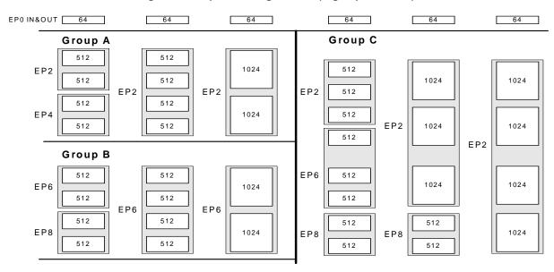
Figure 2. Endpoint Configurations (High Speed Mode)
