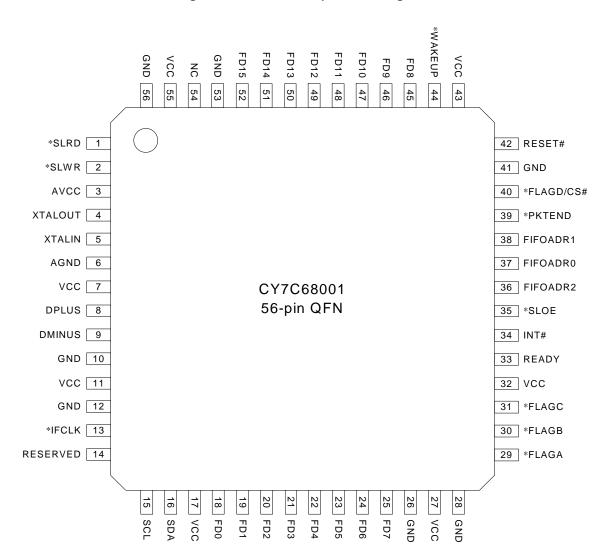
Figure 4. CY7C68001 56-pin QFN Assignment<sup>[7]</sup>
