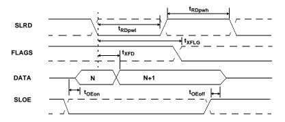
Table 33. Slave FIFO Asynchronous Read Parameters<sup>[20]</sup>
