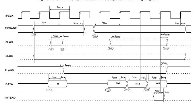
Figure 22. Slave FIFO Synchronous Write Sequence and Timing Diagram<sup>[21]</sup>
