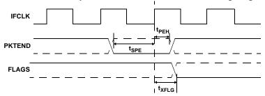
Table 30. Slave FIFO Synchronous Packet End Strobe Parameters, Internally Sourced IFCLK<sup>[19]</sup>
