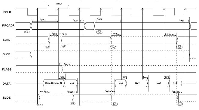
Figure 21. Slave FIFO Synchronous Sequence of Events Diagram
