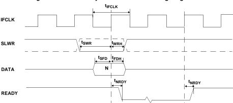
Figure 6. Command Synchronous Write Timing Diagram<sup>[13]</sup>
