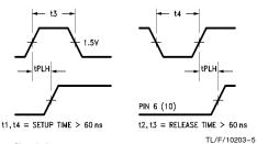
Input to Pin 4 (12) Pins 5 (11) and  $\frac{1}{3}$  (13) = H
