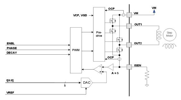
Figure 1. Motor Control Circuitry
