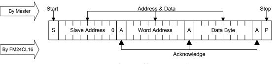
Figure 5. Single Byte Write
