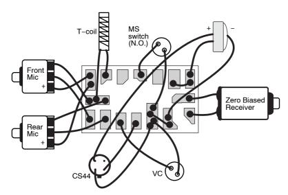
Figure 4. Typical Hearing Instrument Assembly Diagram
