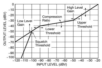
Figure 6. Independent Channel I/O Curve Flexibility
