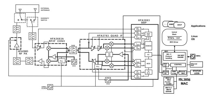
FIGURE 2. ISL36356A-APDK BLOCK DIAGRAM
