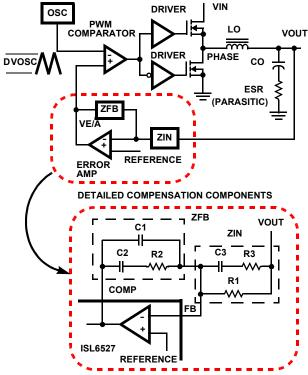
FIGURE 5. VOLTAGE-MODE BUCK CONVERTER COMPENSATION DESIGN
