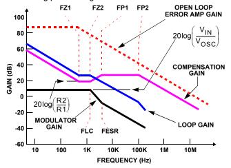
FIGURE 6. ASYMPTOTIC BODE PLOT OF CONVERTER GAIN
