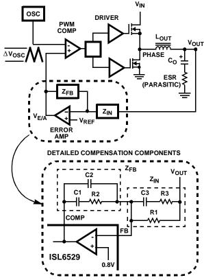
FIGURE 5. VOLTAGE-MODE BUCK CONVERTER COMPENSATION DESIGN
