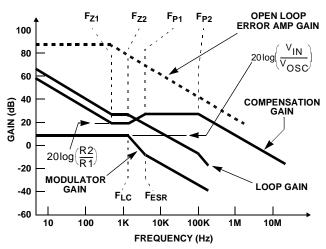
FIGURE 6. ASYMPTOTIC BODE PLOT OF CONVERTER GAIN
