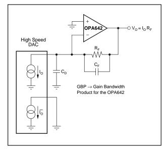
FIGURE 4. Wideband, Low Distortion DAC Transimpedance Amplifier.
