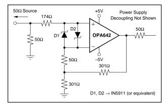
FIGURE 10. Gain of +2 with Input Protection.
