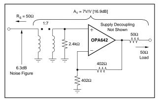
FIGURE 7. Reduced Noise Figure Circuit.
