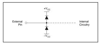
FIGURE 9. Internal ESD Protection.
