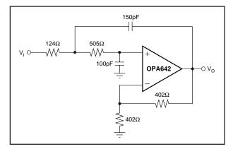
FIGURE 5. 5MHz Butterworth Low Pass Active Filter.
