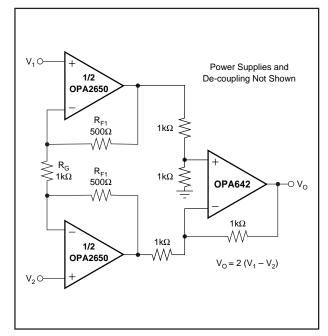
FIGURE 3. Wideband 3-Op Amp Differencing Amplifier.
