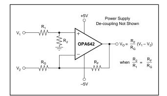
FIGURE 2. High Speed, Single Amplifier Differential Amplifier.
