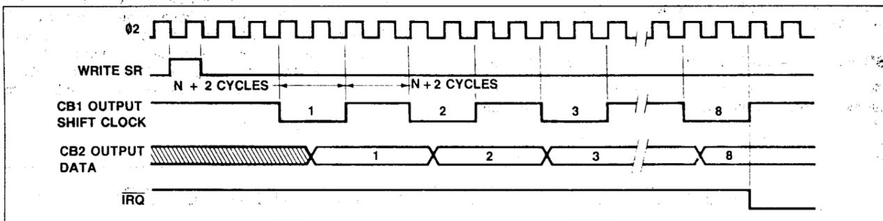
Figure 26. SR Mode 5 — Shift Out Under T2 Control
