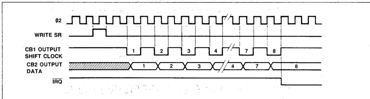
Figure 27. SR Mode 6 — Shift Out Under  $\phi 2$  Control
