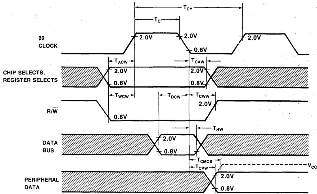
Write Timing Waveforms
