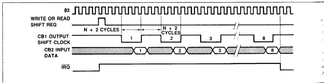
Figure 22. SR Mode 1 — Shift In Under T2 Control
