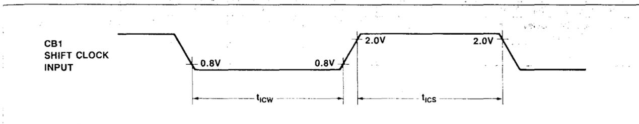
Figure 31h. External Shift Clock Timing
