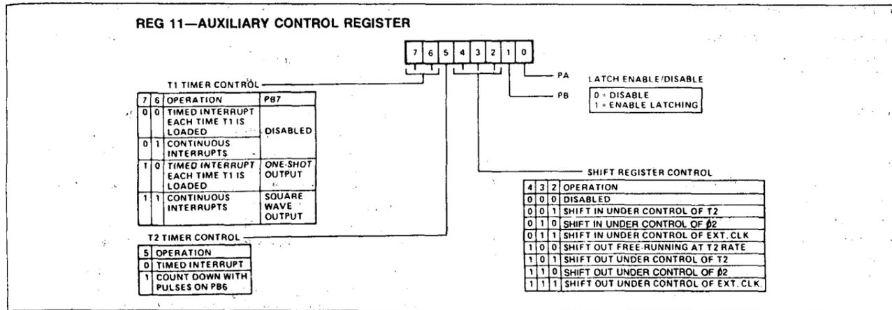
Figure 14. Auxiliary Control Register (ACR)
