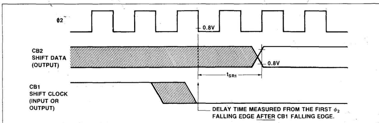
Figure 31f. Timing for Shift Out with Internal or External Shift Clocking
