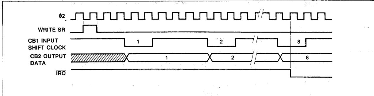
Figure 28. SR Mode 7 — Shift Out Under CB1 Control
