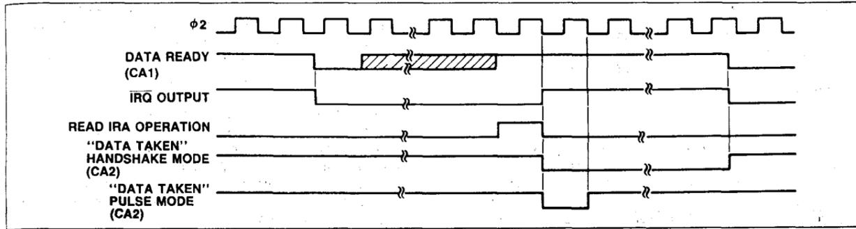
Figure 9. Read Handshake Timing (Port A Only)
