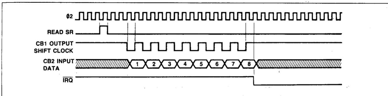
Figure 23. SR Mode 2 — Shift In Center Ø2 Control
