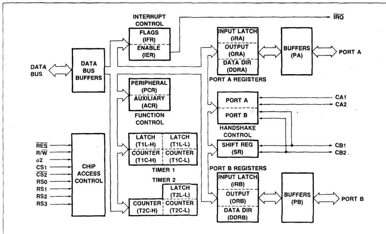
Figure 4. R6522 VIA Block Diagram
