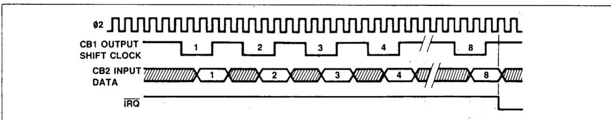
Figure 24. SR Mode 3 — Shift In Under CB1 Control
