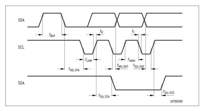
Figure 2 Timing Conditions for the  ${\bf I}^2{\bf C}$  Bus
