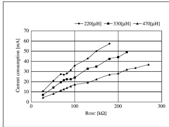
Figure 28. R<sub>OSC</sub> – Current consumption
