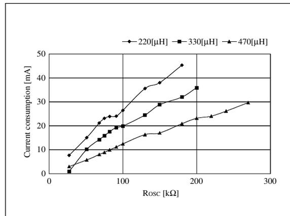
Figure 16. R<sub>OSC</sub> – Current consumption
