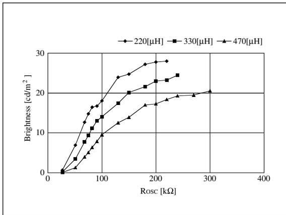
Figure 18. R<sub>OSC</sub> – Brightness
