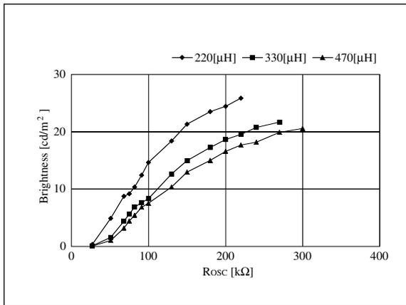
Figure 30. R<sub>OSC</sub> - Brightness
