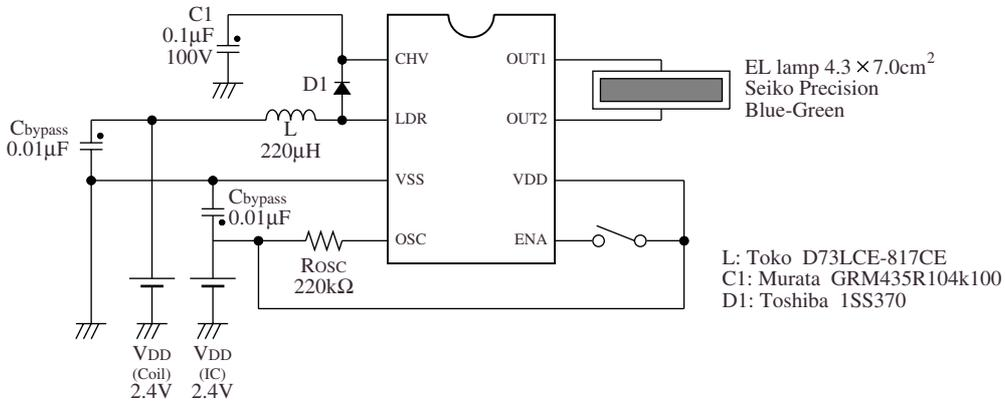
Figure 20. Application circuit
