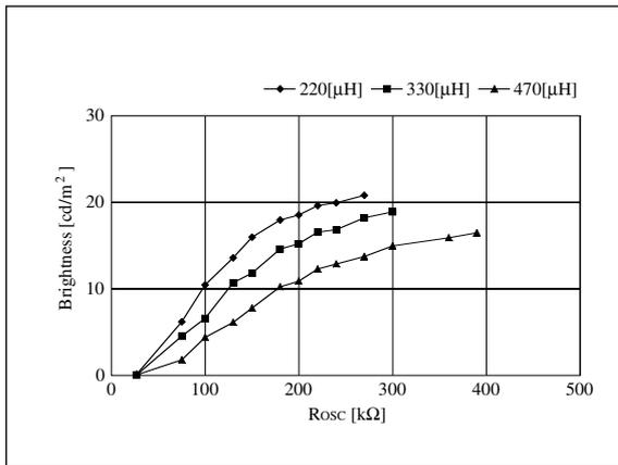
Figure 21. R<sub>OSC</sub> – Brightness
