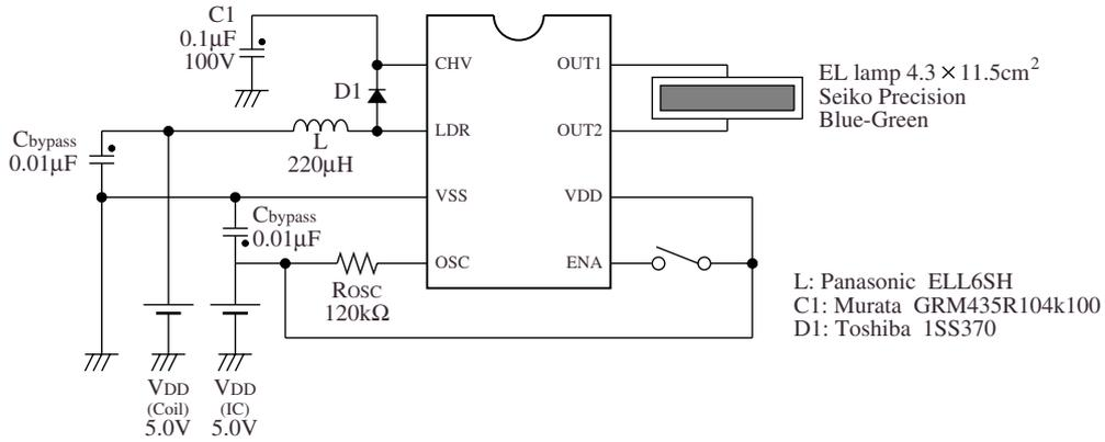
Figure 41. Application circuit
