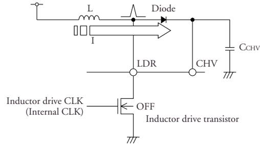
Figure 7. Boost circuit (transistor OFF)
