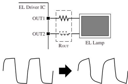
A shielded (3-pin type) EL display is effective in preventing noise between the EL display and other components. Also, the piezoelectric effect can be prevented by avoiding potentials on plane surfaces, such as VDD or ground planes.
