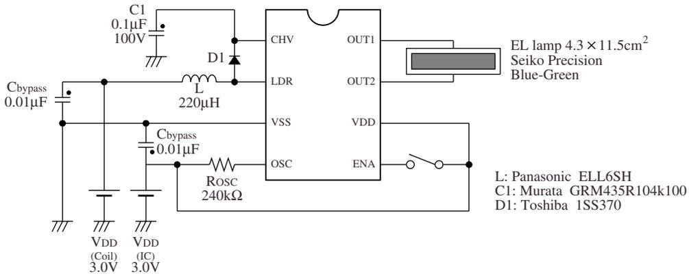
Figure 35. Application circuit
