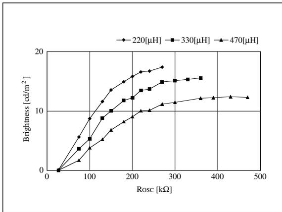
Figure 24. R<sub>OSC</sub> - Brightness
