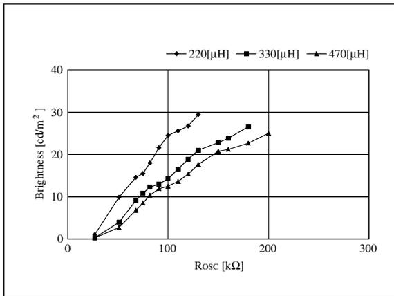
Figure 42. R<sub>OSC</sub> – Brightness
