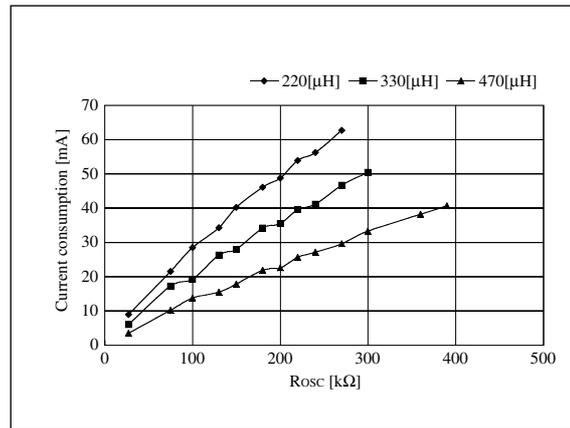
Figure 22. R<sub>OSC</sub> – Current consumption
