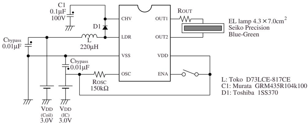
Figure 9. Output waveform adjustment circuit
