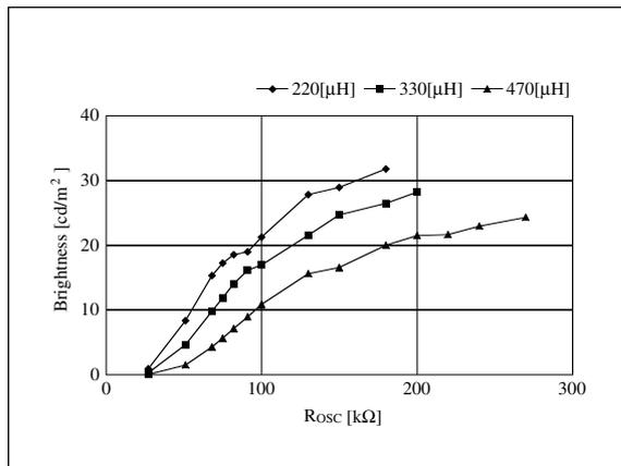
Figure 15. R<sub>OSC</sub> – Brightness
