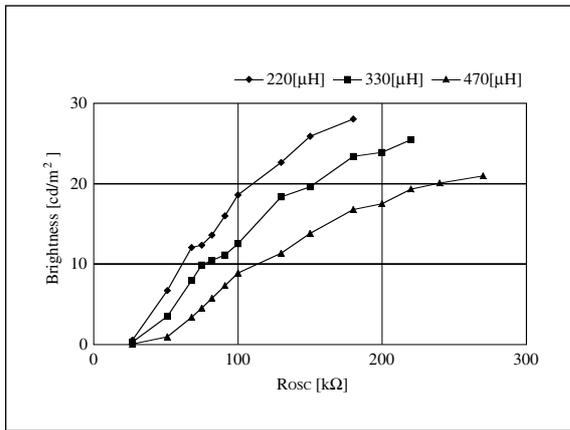
Figure 27. R<sub>OSC</sub> – Brightness
