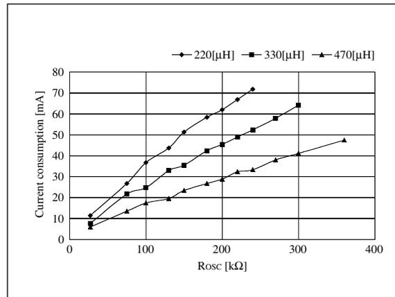
Figure 34. R<sub>OSC</sub> – Current consumption
