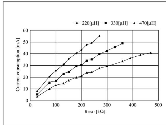
Figure 25. R<sub>OSC</sub> - Current consumption
