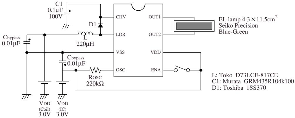
Figure 32. Application circuit
