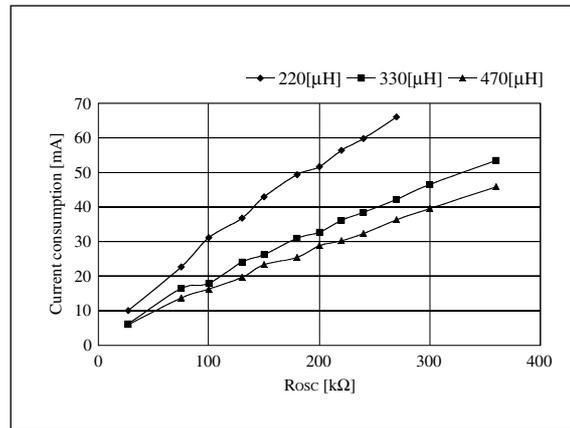
Figure 37. R<sub>OSC</sub> – Current consumption
