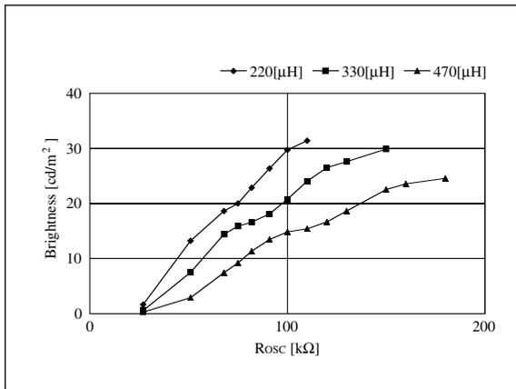
Figure 39. R<sub>OSC</sub> - Brightness
