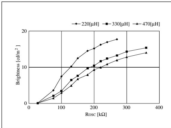
Figure 36. R<sub>OSC</sub> – Brightness
