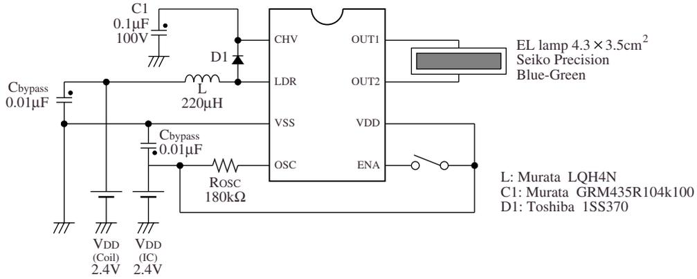
Figure 17. Application circuit
