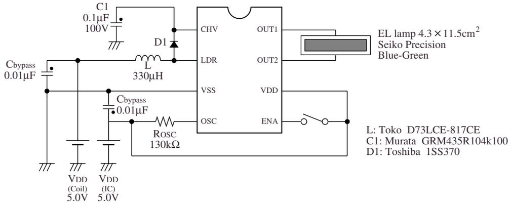
Figure 38. Application circuit
