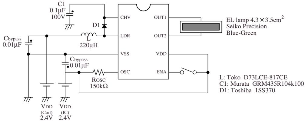
Figure 14. Application circuit
