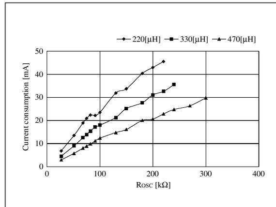
Figure 19. R<sub>OSC</sub> – Current consumption
