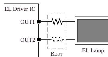
The reduction in  $C_{CHV}$  ringing noise is the same in both cases, but making  $R_{OUT}$  larger does have an unfavorable result on efficiency. Inserting  $R_{CHV}$ , however, is an effective way of reducing only the  $C_{CHV}$  ringing noise.
