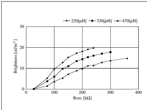
Figure 33. R<sub>OSC</sub> – Brightness
