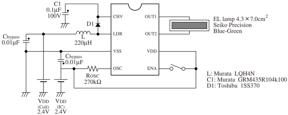
Figure 23. Application circuit
