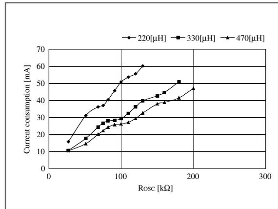
Figure 43. R<sub>OSC</sub> – Current consumption
