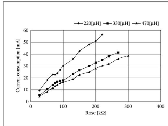
Figure 31. R<sub>OSC</sub> - Current consumption
