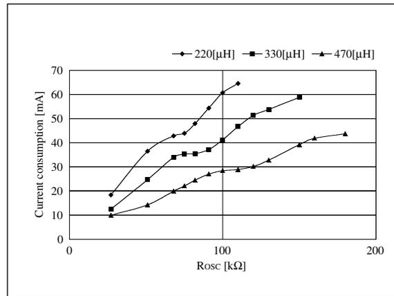
Figure 40. R<sub>OSC</sub> - Current consumption
