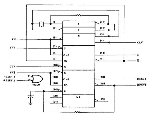
FIGURE 1. CLOCK AND RESET GENERATION FOR MICROPROCESSOR-BASED SYSTEM
