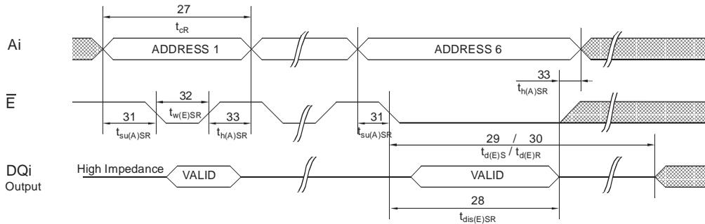
u:  $\bar{W}$  must be HIGH when  $\bar{E}$  is LOW during the address sequence in order to initiate a nonvolatile cycle.  $\bar{G}$  may be either HIGH or LOW throughout. Addresses 1 through 6 are found in the mode selection table. Address 6 determines whether the U635H64 performs a STORE or RECALL.
