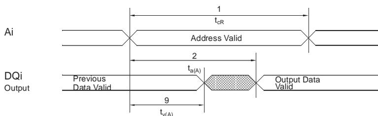
Read Cycle 2:  $\bar{G}$ -,  $\bar{E}$ -controlled (during Read cycle:  $\bar{W} = V_{IH}$ )<sup>g</sup>
