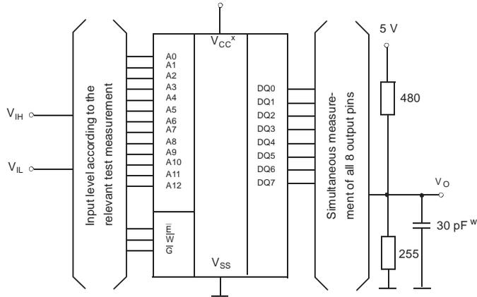
w: In measurement of  $t_{dis}$ -times and  $t_{ben}$ -times the capacitance is 5 pF.
