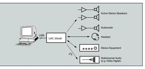
Fig. 1: Typical applications for the UAC 355xB
