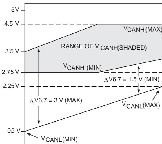
NOTE: Valid voltage range of  $V_{CANH}$  for sensing dominant bus state as  $V_{CANL}$  varies. TXD = LOGIC 0
