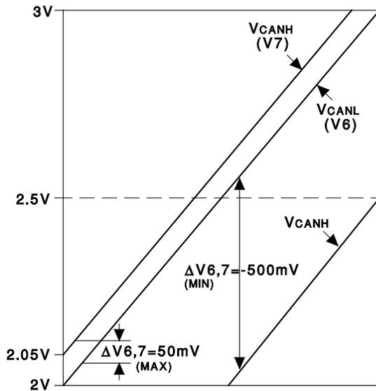
NOTE: Valid output of CANH, CANL during recessive state transmission. TXD = LOGIC 1
