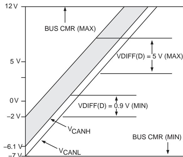
NOTE: Valid voltage range of  $V_{CANH}$  for sensing dominant bus state as  $V_{CANL}$  varies over bus common mode range. TXD = LOGIC 0
