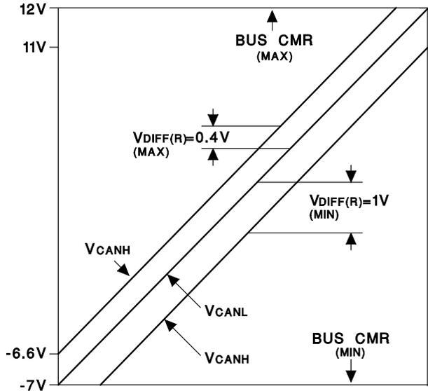
NOTE: Valid voltage range of  $V_{CANH}$  for sensing dominant bus state as  $V_{CANL}$  varies over bus common range mode. TXD = LOGIC1
