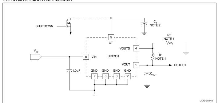
Note 1: R1 and R2 for adjustable version only. For 3.3V and 5V versions connect VOUT to VOUTS. See Pin Descriptions.
