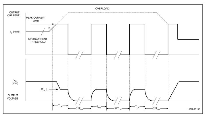
Figure 1. UCC381 short circuit timing.
