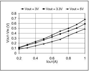
Figure 2. Typical dropout vs. load current.
