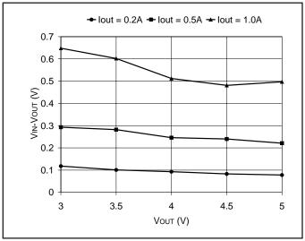
Figure 3. Typical dropout voltate vs. I<sub>OUT</sub> and V<sub>OUT</sub>.
