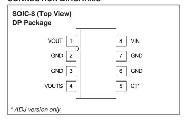
The UCC381 can be shutdown to  $25\mu A$  (max) by pulling the CT pin low.
