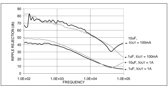
Figure 5. Ripple rejection vs. frequency.
