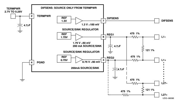
Figure 1. Low-Voltage Differential Discrete Resistor Stack
