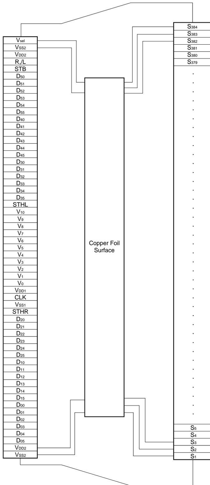
**Remark** The  $V_{sel}$  pin is internally pulled up.
