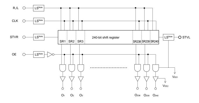
Note LS (level shifter): Shifts 5 V/3.3 V CMOS level and VDD2-VEE1 level.
