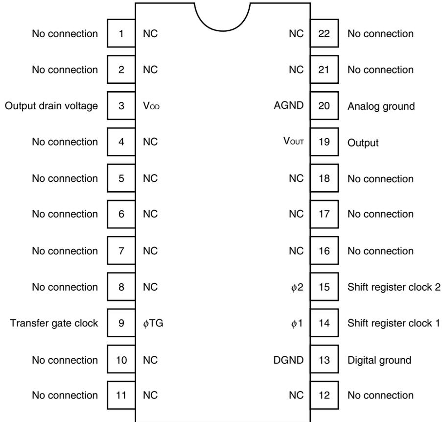
★ **Caution** Connect the No connection pins (NC) to GND.
