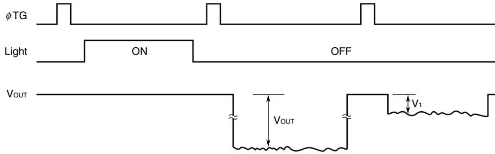
$$IL (\%) = \frac{V_1}{V_{OUT}} \times 100$$
