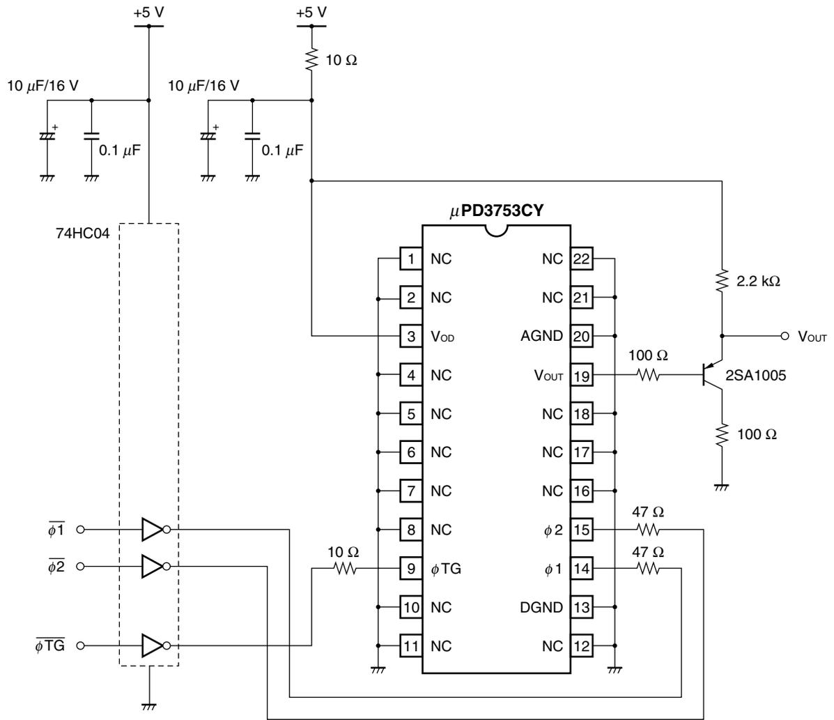
★ **Caution** Connect the No connection pins (NC) to GND.
