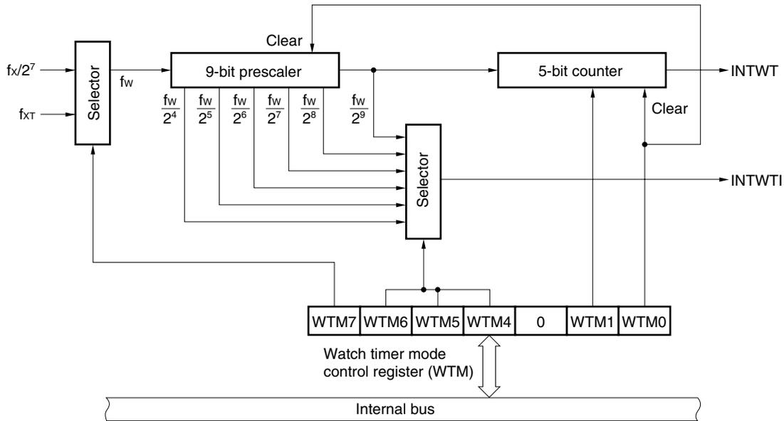
Figure 5-6. Block Diagram of Watchdog Timer
