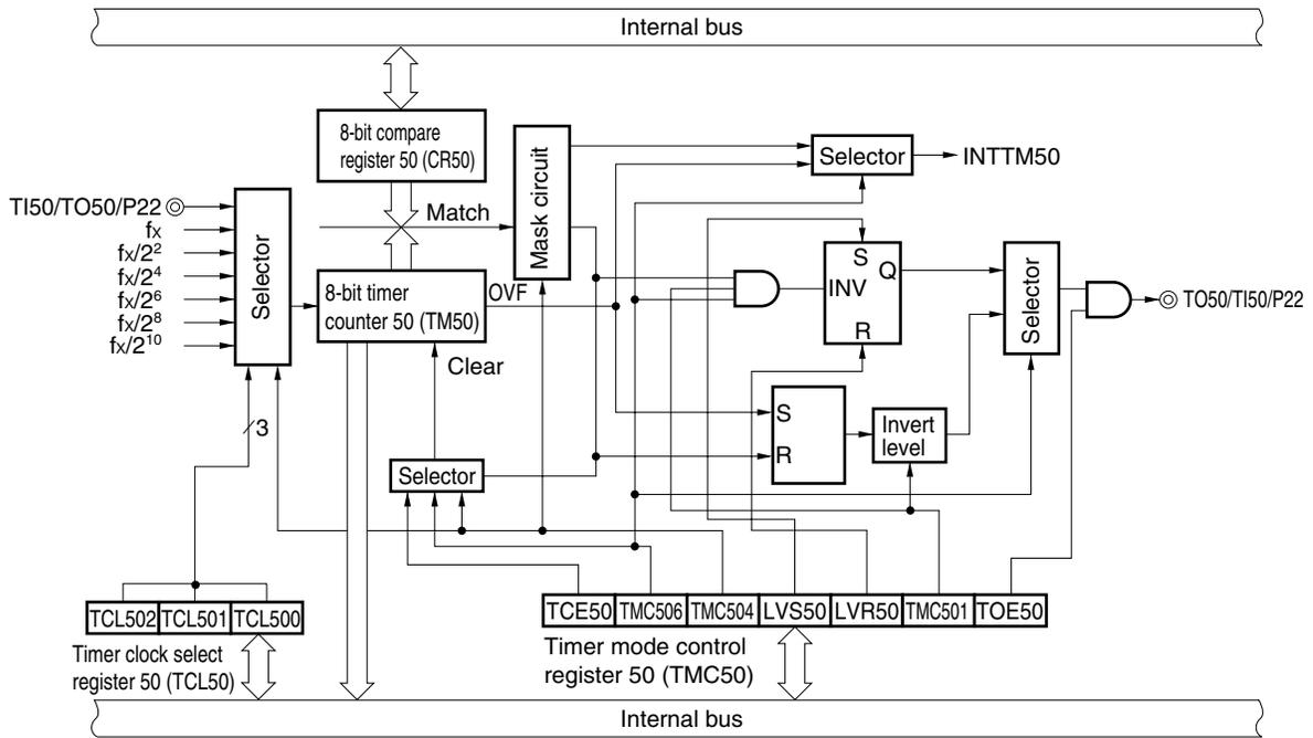
Figure 5-4. Block Diagram of 8-bit Timer/Event Counter 51
