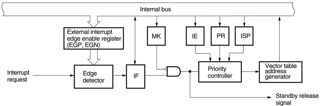
Figure 6-1. Basic Configuration of Interrupt Function (2/2)
