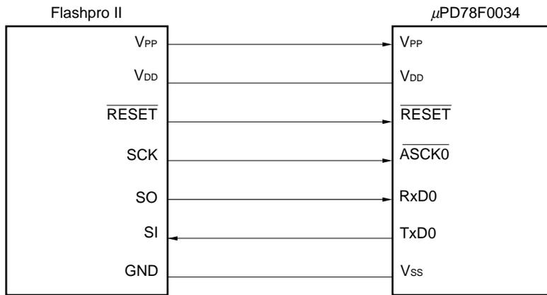
Figure 4-4. Connection of Flashpro II Using Pseudo 3-Wire Serial I/O Method
