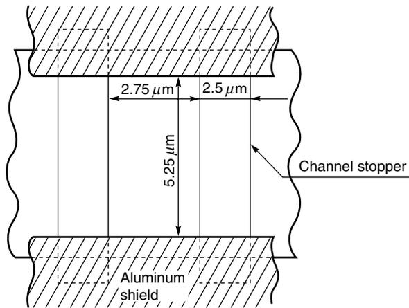
PHOTOCELL ARRAY STRUCTURE DIAGRAM (Line spacing)
