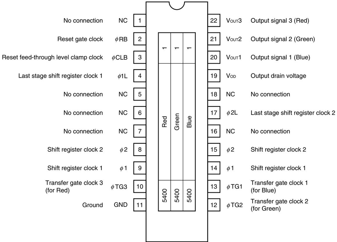
**Caution** Connect the No connection pins (NC) to GND.
