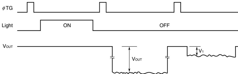
$$\text{IL (\%)} = \frac{V_1}{V_{\text{OUT}}} \times 100$$
