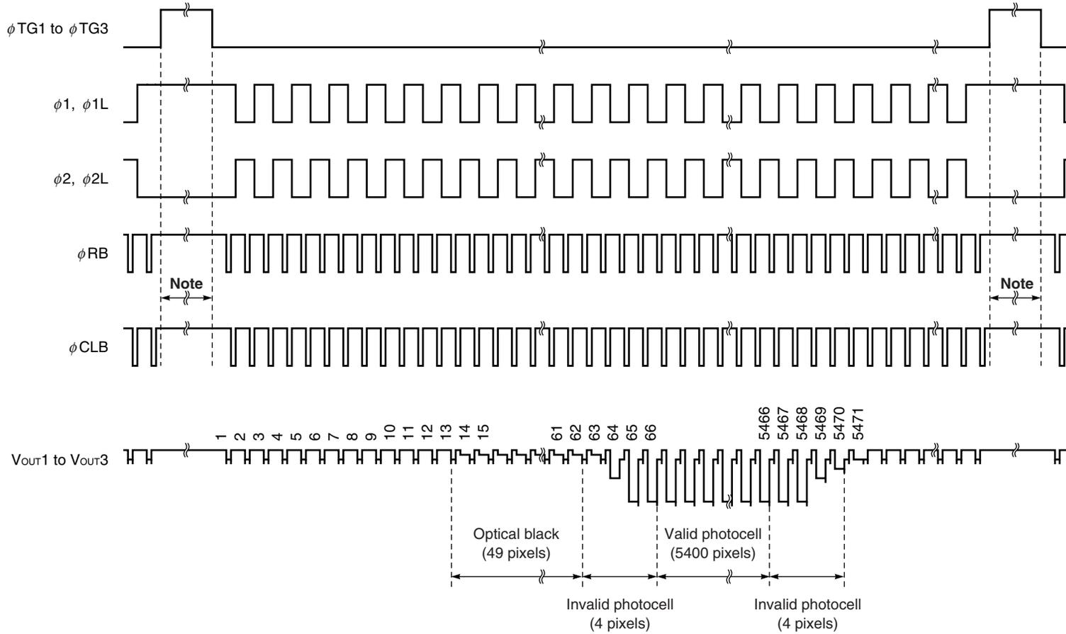
**Note** Set the  $\phi$ RB and  $\phi$ CLB to high level during this period.
