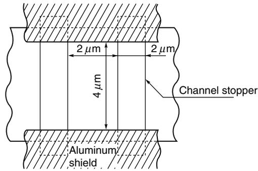
PHOTOCELL ARRAY STRUCTURE DIAGRAM (Line spacing)
